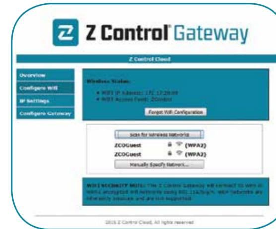
5. After one minute or so, verify that the flashing blue "Internet and Z Control® Cloud Light" on the Gateway has turned to solid blue. If it doesn't, then the connection was unsuccessful. The Gateway will require a reset by holding the Link button during Power Up for 10 seconds. This will force the Gateway to return to Wireless Access Point mode, as described above. *The most common reason the Gateway didn't connect successfully is that the pass phrase was entered incorrectly.*
